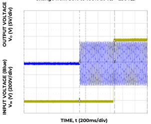
Figure 6. Typical Start-up ( $V_{IN}$  = 230 $V_{ac}$ , Full load).
