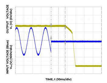
Figure 7. Typical Hold-up waveforms – all except ..Z02A version ( $V_{\text{IN}}$  = 115V, 100% load).
