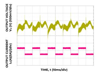
Figure 4. Transient Response to Dynamic Load Change from 50% to 100% at V<sub>IN</sub> = 230V<sub>ac</sub>.
