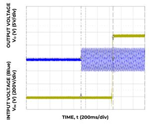
Figure 5. Typical Start-up ( $V_{IN}$  = 115 $V_{ac}$ , Full Load).
