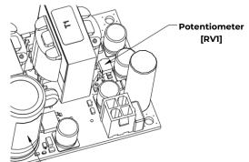
Fig. 11. Diagram showing location of the potentiometer used to adjust the power supply output voltage.
