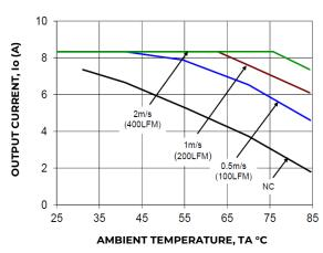
Figure 2. Derating Output Current versus Ambient Temperature and Airflow. Data shown for 115VAC in, at 230VAC in derating is the same or better. For derating at other input voltages, consult the OmniOn Technical representative.
