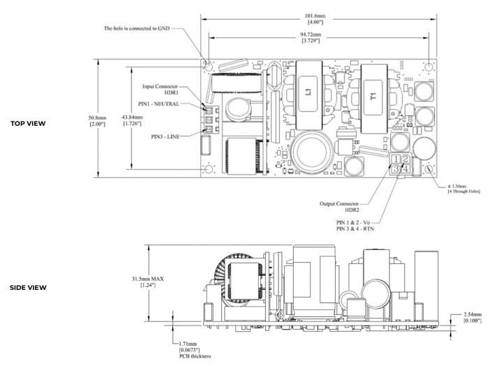
Minimum clearance of 6mm required on bottom of the unit.
