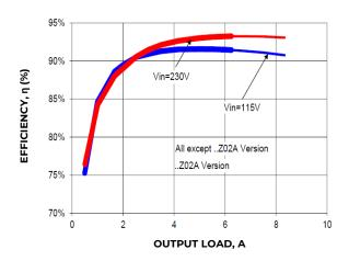
Figure 1. Power Supply Efficiency versus Output Current.
