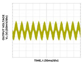
Figure 3. Typical output ripple and noise  $(V_{IN} = 230V_{ac}, 100\% \text{ load }).$
