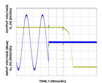
Figure 10. Typical Hold-up waveforms -..Z02A version ( $V_{\rm IN}$  = 230V, 100% load).
