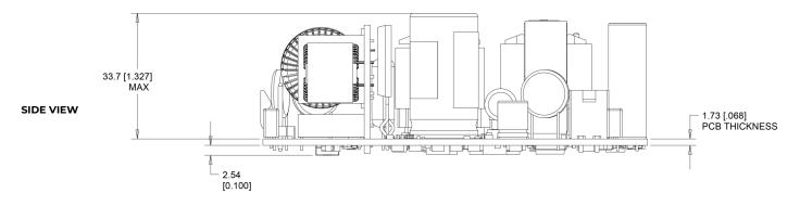
Minimum clearance of 6mm required on bottom of the unit.
