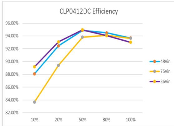
Figure 1: Power Supply Efficiency Versus Output Current
