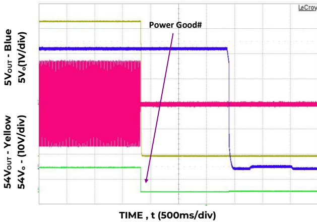
Figure 15. Turn-OFF at full load, V IN =230V AC
