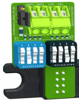
Jumper pins 1-2 Pass through
