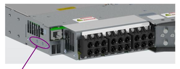
Wire size: 6AWG SCREW MCH #10-32 Lug landings: #10 double hole on 0.625 inch center Torque: 30±1.5In-lb. (3.4Nm)
