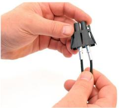
Step 4: Install pin separator into connector chassis (push until the retainer "snaps" into place)
