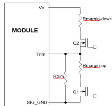
**Figure 37. Circuit Configuration for margining Output voltage.**
