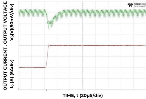
Figure 28. Transient Response to Dynamic Load Change from 50% to 100% at 12Vin,  $C_{out} = 4x47\mu F + 1x330\mu F$   $C_{Tune}=1800pF$ ,  $R_{Tune}=300$
