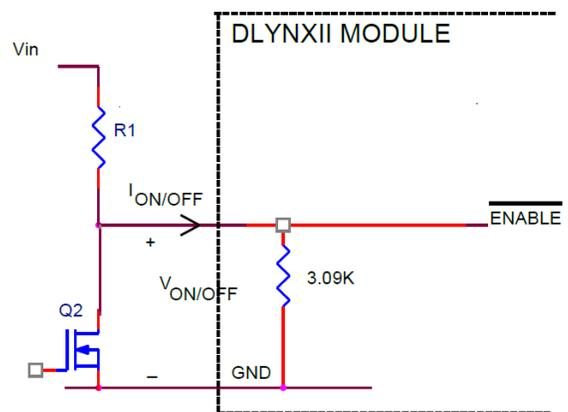
Figure 34. Circuit configuration for using negative On/Off logic.
