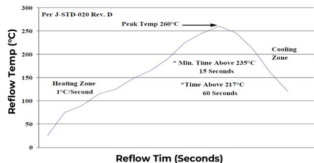
Figure 44. Recommended linear reflow profile using Sn/Ag/Cu solder.
