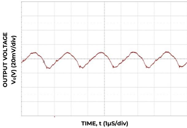
Figure 27. Typical output ripple ( $C_o=7x22\mu F$  ceramic,  $V_{IN} = 12V$ ,  $I_o = I_{o,max}$ ).
