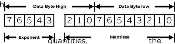
module supports the “Linear” data format among the three data formats supported by PMBus. The Linear Data Format is a two byte value with an 11-bit, two’s complement mantissa and a 5-bit, two’s complement exponent. The format of the two data bytes is shown below:
