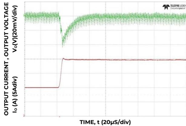
Figure 16. Transient Response to Dynamic Load Change from 50% to 100% at 12Vin,  $C_{out} = 7 \times 47\mu\text{F} + 2 \times 330\mu\text{F}$  CTune=3900pF, RTune=300
