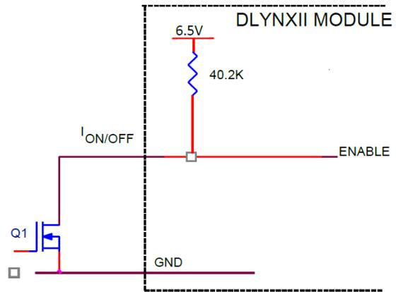
Figure 33. Circuit configuration for using positive On/Off logic
