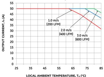
Figure 22. Output Current Derating for the Base plate QSD (V)W050A0B-H with a 1.0" Heat Sink and Transverse Airflow
