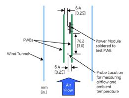
The power modules operate in a variety of thermal environments and sufficient cooling should be provided to help ensure reliable operation. Thermal considerations include ambient temperature, airflow, module power dissipation, and the need for increased reliability. A reduction in the operating temperature of the module will result in an increase in reliability.
