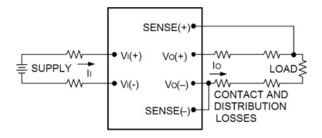
Figure 15. Circuit Configuration for remote sense.
