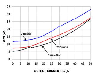
Figure 2. Typical Converter Loss vs. Output Current.
