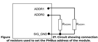
The user must know which I<sup>2</sup>C addresses are reserved in a system for special functions and set the address of the module to avoid interfering with other system operations. Both 100kHz and 400kHz bus speeds are supported by the module.
