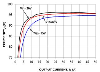
Figure 1. Typical Converter Efficiency vs. Output Current.
