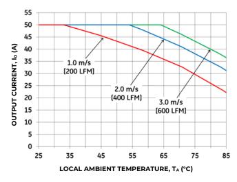
Figure 21. Output Current Derating for the Base plate QSD (V)W050A0B-H with a 0.5" Heat Sink and Longitudinal Airflow from Vout to Vin; Vin=48V.
