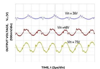
Figure 3. Typical Output Ripple and Noise,  $I_o$  =  $I_{o,max}$ , Co = Co,min
