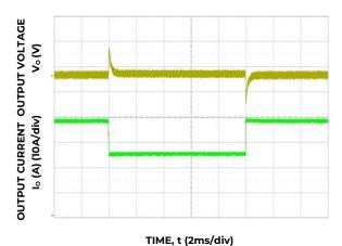
Figure 4. Typical Transient Response to 1.0A/µs Step Change in Load from 50% to 75% to 50% of Full Load, Co=470µF and 48 Vdc Input.
