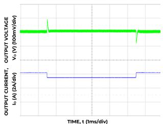
Figure 4. Transient Response to 0.1A/µS Dynamic load Change from 50% to 75% to 50% of full load, V<sub>in</sub>=24V,
