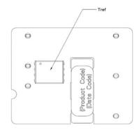
Figure 16. T<sub>ref</sub> Temperature Measurement Location.
