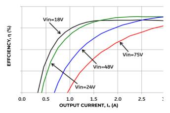
Figure 1. Converter Efficiency versus Output Current.
