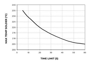
Figure 21. Time Limit, T  $_{\mbox{\scriptsize lim}}$ , Curve Above 205°C Reflow .
