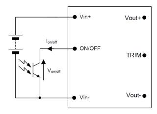
Figure 10. Circuit configuration for using Remote On/Off Implementation.
