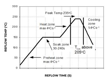
Figure 20. Recommended Reflow Profile for Sn/Pb solder.
