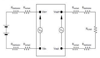
Figure 9. Output Voltage and Efficiency Test Setup.
