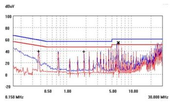
Figure 18. EMC signature using above filter.
