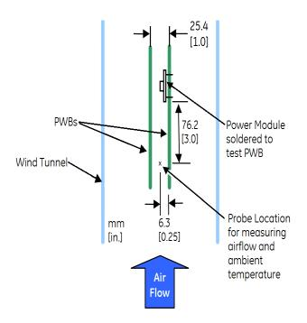
Figure 13. Thermal Test Setup.
