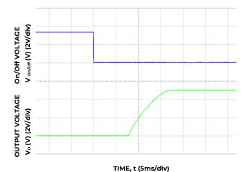
Figure 5.Typical Start-up Using Remote On/Off, negative logic version shown ( $V_{IN}$  = 24V or 48V,  $I_0$  =  $I_0$ ,  $_{max}$ ).
