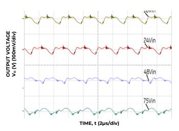
Figure 3. Typical output ripple and noise (  $I_{\text{O}}\text{= }I_{\text{O}\text{, }\text{max.}}\text{)}$
