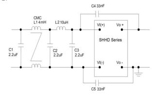
Figure 17. Suggested Configuration for EN55032 Class B.
