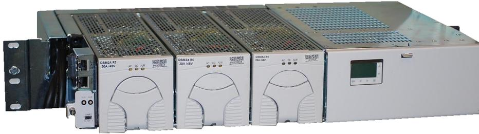
The CPS6000 comes in a 19" or 23" shelf configuration. Install the shelf with a minimum gap of 3/4 inch above and below to allow proper airflow. Attach the CPS shelf to the frame using a minimum of four (two on each side) of the 12-24 screws included with the shelf.
